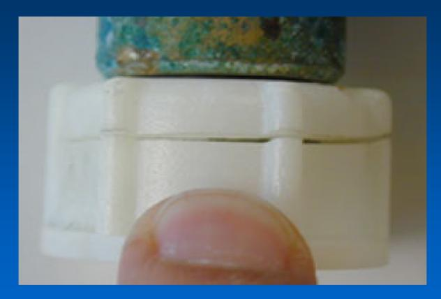
Failure resulting from ignoring installation instructions
