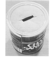
Figure 6-16 PE coffee can cover used beyond its intended service; a rectangular hole was cut in th center, leading to cracks at the corners ([1] Fig. 3, reproduced with permission)
