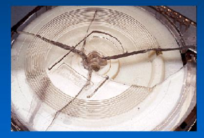
Branching Look for cracks on the failed part. The cracks that end before they reach the edge of the part are AWAY from the origin. These cracks typically exhibit branching.
