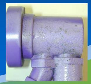
Degradation from prolonged contact with Gasoline
