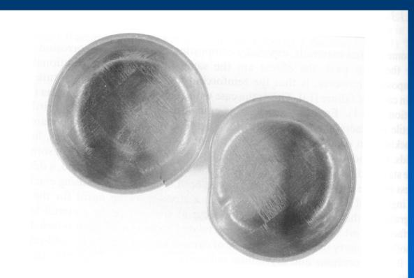
Figure 6-8 IPS salad bowls deformed and cracked due to washing in dishwasher
